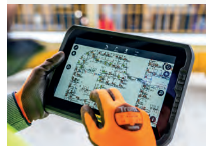
Trimble Field Points generates accurate setting out positions for all the required points
